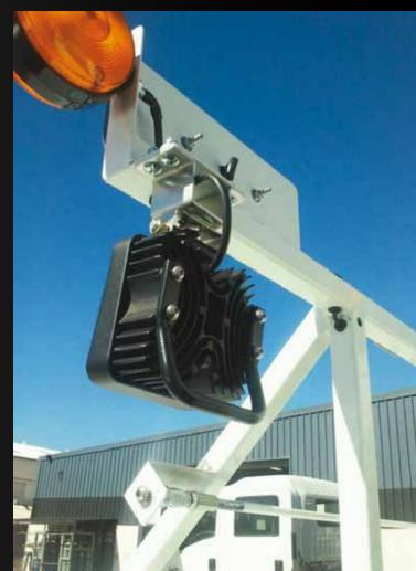
The Low Voltage Work Lamp Swivel base is designed to work with all work lamps which have a single stud mount.
